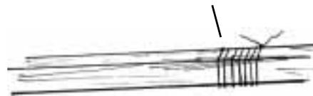
If the fibers start to split off, quickly wrap that place with string, keeping the fibers intact. Continue bending gently.
