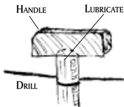
The handle can be of any material. There should be a shallow hole in the handle to fit the drill. Lubricate this. It does not need friction.
