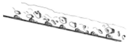
First they screen and size the material. Then they use the very high specific gravity of gold to separate it from the other rocks. Water and the ore are kept in motion down the sluice box. Gold and black
