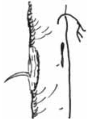
Split a thin piece of birch from a block. Saw another piece identical in size to the split one. Try bending them. Which bends best?
