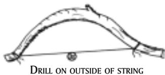
Twist the drill into the string of the bow. The drill should be on the outside of the string, not
