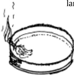
There are three parts to a traditional lamp: the container, the wick and the fuel. The fuel is from seals, moose, whales, bears, fish, etc. The lamp itself must be of a material that won't burn such as rock, clay, sea shells or metal. The wick was traditionally of certain mosses, but cotton replaced moss long ago. The wick
