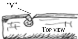
Flatten the bottom piece of dry willow or alder on two sides. With a knife or drill, make an indentation, and then cut a "V" up to the middle of that indentation.
